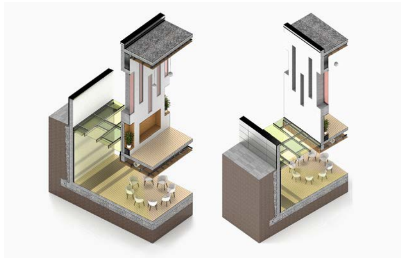
Axonometric Wall Section Showing Tinted Glass
